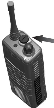
**3** To attach, remove the accessory cover by unscrewing the locking screw anti-clockwise (leave cover secured under antenna as this provides a waterproof seal). Attach accessory plug by locating over the socket. Carefully tighten the locking screw clockwise until finger tight (do not tighten with a screwdriver etc).
